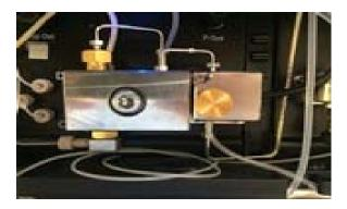
b. Then put a check in the purge box and this window will pop up. Start the purge – the purge process has a built in timer. If there is still visible air in the lines, purge a second time. Once the timer has elapsed, the purge button will go from green back to gray. Be sure to <u>CLOSE THE PURGE VALVE!</u>
