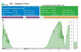
Don Colliver shared the photo (left) which shows the dramatic reduction in electricity output from the solar system at the UK Horticulture Farm during the eclipse last week.
