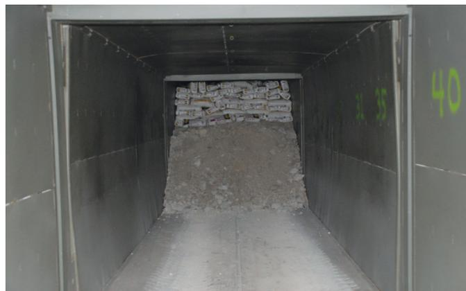
Photograph of the gob pile in the shock tube.
